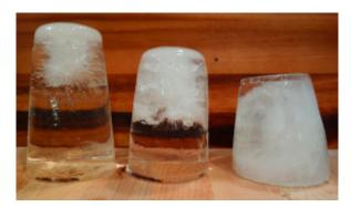
These 3 pieces of ice are sitting top down. All used filtered water. Left: there was a small amount of unfrozen water in the bottom. Fractures and bubbles had started to form. There is plenty of usable clear ice in this piece. Center: the ice has frozen
